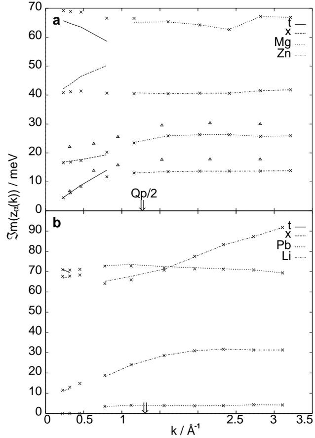
Figure 2. The imaginary parts of eigenvalues for liquid metallic alloys: (a)  $\text{Mg}_{70}\text{Zn}_{30}$ ; (b)  $\text{Li}_4\text{Pb}$ . Triangles show the spectrum of transverse collective excitations found for amorphous  $\text{Mg}_{70}\text{Zn}_{30}$  at room temperature (from Ref. [13]). All other settings are as in Figure 1.
