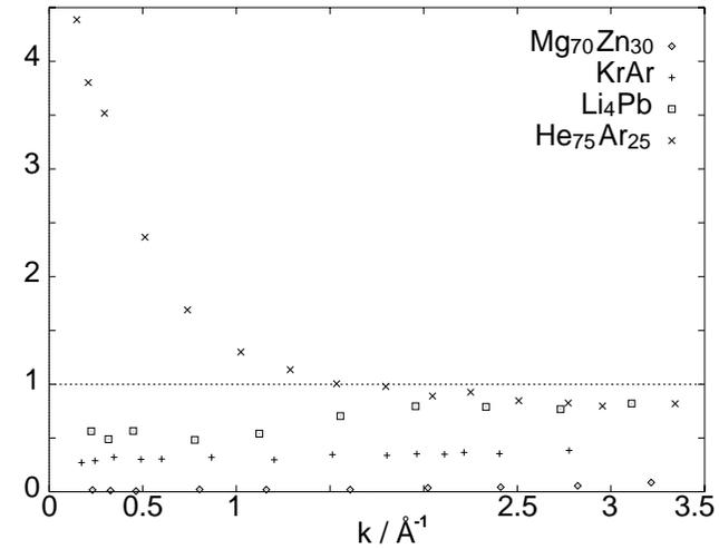
Figure 3. Left side of condition (7) as a function of  $k$  for:  $\text{Mg}_{70}\text{Zn}_{30}$ , Kr-Ar,  $\text{Li}_4\text{Pb}$ , and  $\text{He}_{75}\text{Ar}_{25}$ . Reduced units  $k_B T = 1$ ,  $\bar{m} = 1$ , and  $k_{\min} = 1$  are used, where  $k_{\min}$  is the smallest  $k$ -value available in molecular dynamics.
