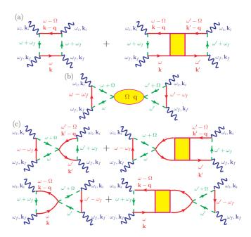
FIG. 4. (Color online) Diagrams for the renormalized fourparticle correlation function  $\chi^{(4)}$ . Panel (a) total direct resonant scattering, (b) full exchange resonant scattering, and (c) partial exchange resonant scattering processes. Explicit  $E_h$  dependence of the core-hole propagator is not shown.
