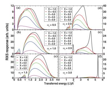
FIG. 9. (Color online) Systematic evolution of the RIXS response as a function of transferred energy  $(\Omega)$  for six incident photon energies from the bottom of the upper Hubbard band:  $\omega_i = 0.5$  (a) to the top of the upper Hubbard band  $\omega_i = 3.0$  (f). The dispersive nature of the high-energy peak (Mott gap excitation) is noticeable. All other parameters are the same as in Fig. 7.
