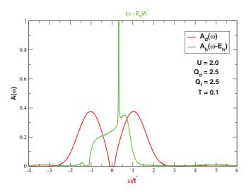
FIG. 6. (Color online) Spectral function for the d hole,  $A_d(\omega)$ , and the core hole,  $A_h(\omega - E_h)$ . For  $A_h(\omega - E_h)$ , the frequency is measured with respect to the core-hole energy,  $E_h$ , as shown in the top horizontal axis.
