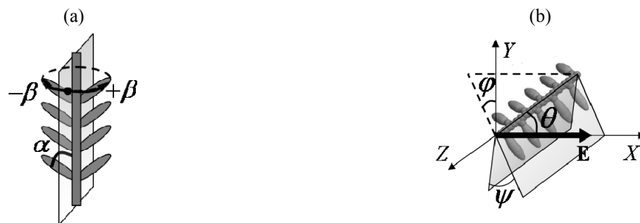
Figure 1. (a) Orientation distribution of chromophores inside an oligomer. (b) Spatial orientation of an oligomer with respect to the electric vector of the light \mathbf{E} ; \theta , \phi and \psi are the three Euler angles, see the text for details.
